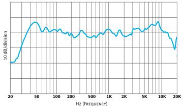
Measured in a free-field anechoic environment using a swept one-third octave input.
