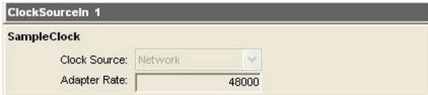
Figure 8. Clock Source information for CobraNet devices as seen in ASIControl.
